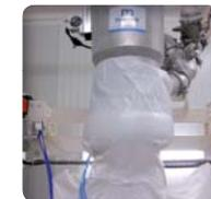
▶ **Inflating seal** to ensure dust containment for a clean workplace
