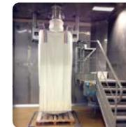
▶ **Suspended structure:** facilitates floor cleaning
