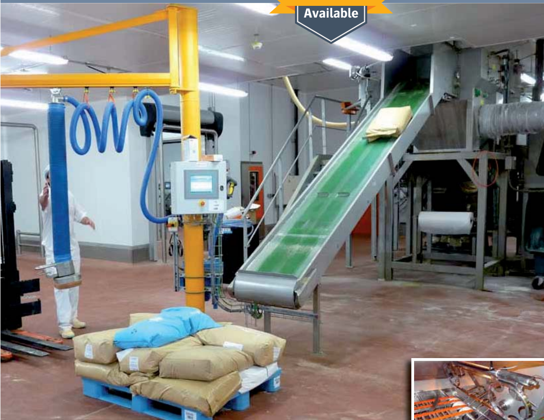
➤ The belt conveyor transports the bag directly to the band-saw cutting system
