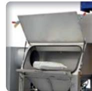
▶ **The gas cylinders** allow the heavy-duty door to be lifted with ease and firmly maintained in an open position
